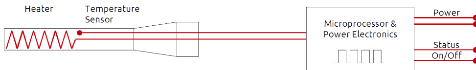
Figure 4. Functional diagram of the HPS-1 heater system
